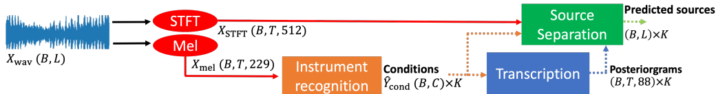
Figure 1. The proposed Jointist framework. Our actual framework can transcribe/separate up to 39 different instruments as defined in Table 7 of Appendix. B : batch size, L : audio length, C : instrument classes, T : number of time steps, K : number of predicted instruments. Dotted lines represent iterative operations for K times. Best viewed in color.
